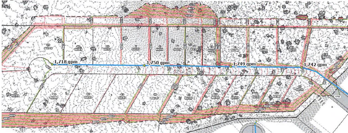
Figure 4 – Available Fire Flow at 20 psi
