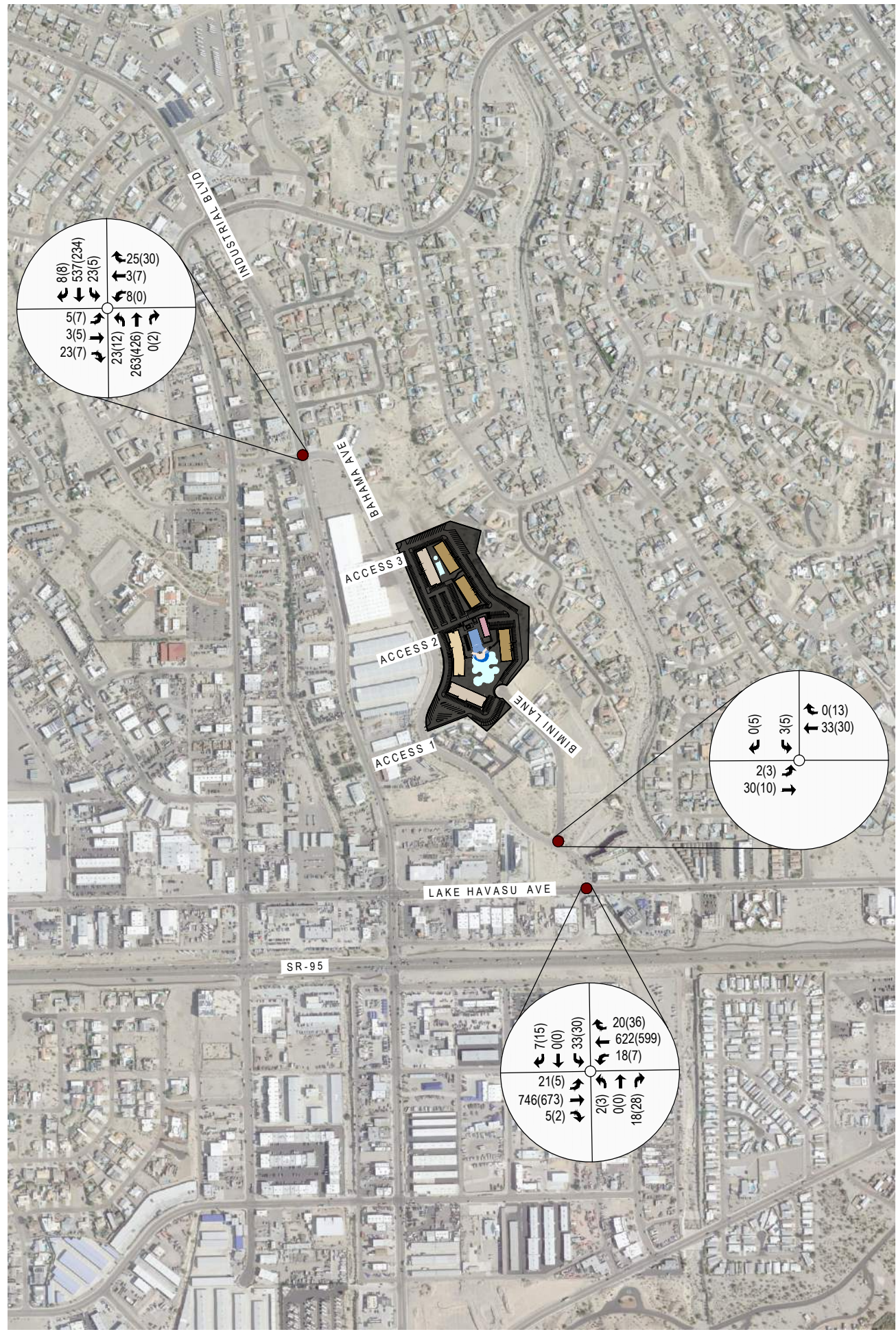
BAHAMA AVE RESORT FIGURE 5 -2030 FULL BUILD-OUT YEAR TRAFFIC VOLUMES XX(XX) = AM(PM) PEAK HOUR TRAFFIC VOLUMES
